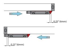
5. After mounting location has been determined and all preparations complete, hand tighten reader head mounting screws and apply light pressure to the reader head, so it firmly touches red plastic shipping bracket. Fully tighten the screws while maintaining uniform pressure on the reader head.
