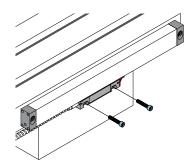
**b** Reader head comes with pretapped M4 holes at the bottom. You can use this feature to attach the included mounting bracket to the scale. This option is typically used for Y axis on the Milling machine and Z axis on lathes.
