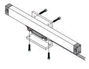
Remove the screw(s) holding shipping bracket to the encoder scale body. Do not remove shipping bracket from the reader head yet. Move machine axis to the dead stop on one end and mark reader head location. Gently slide reader head towards the same end and then slide it 1/4" (6mm) back to allow for travel reserve (safety factor). Mark reader head position on the moving axis. Repeat for the other end. Make sure to avoid over-travel! Obtain larger size scale if necessary.
