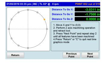
The graphic display of the DR400 series is particularly useful for verifying programmed bolthole pattern inputs before machining. Moreover, the DR400's real-time graphics eliminate guesswork by displaying the exact drawing of the feature you are machining.
